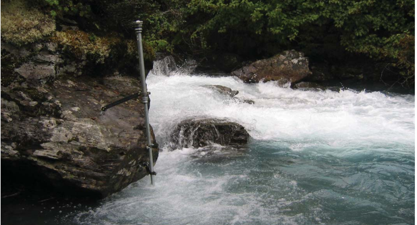
View of one of the stream gauges installed to measure the hydrology of Allison Creek
