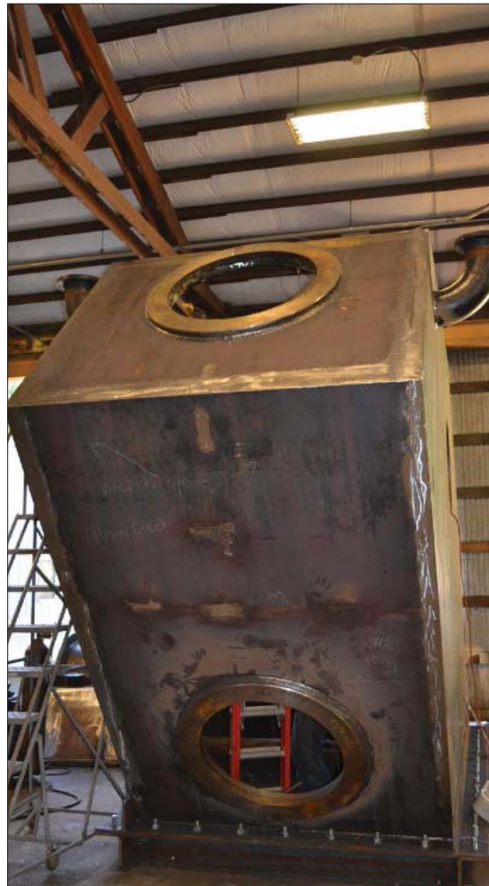
Opposite Left, local contractors just past the rock outcrop on the lower access road Opposite top, lower access road Opposite bottom, the completed Pelton Wheel Top, crews clearing the site of the Power House Above, crews clearing lay down area Right, housing unit where spear nozzles from the penstock will enter; spear nozzles control the quantity of water being shot at the turbine wheel
